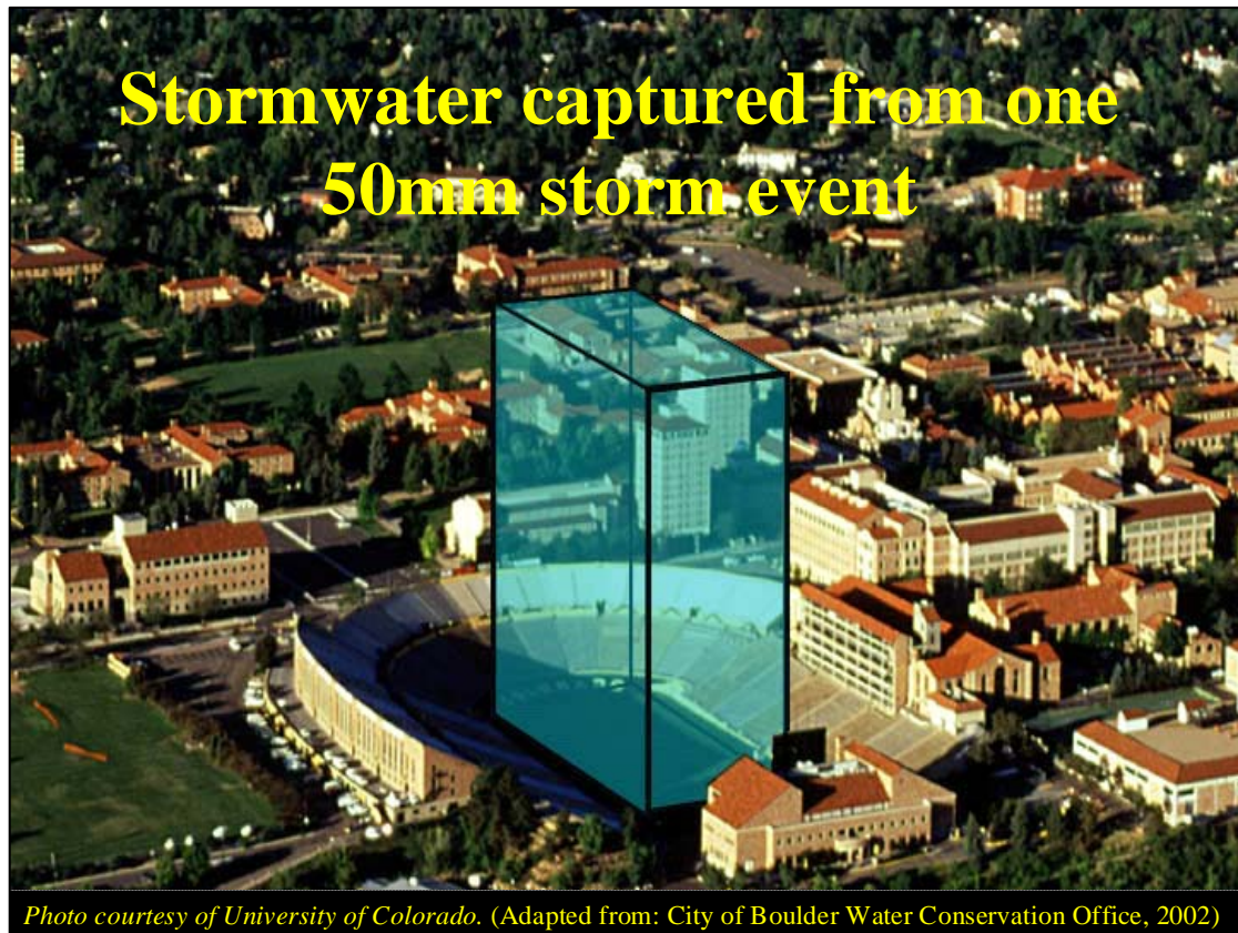
Figure 13 Boulder's canopy cover is responsible for retaining 374 megalitres of stormwater during a 50 mm storm event, roughly equivalent to the volume a 20-story building the size of a football field.
